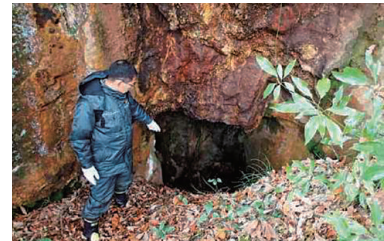
Contact of rainwater seeping underground with mineral ore may generate acid water that contains heavy metals. Monitoring water from surrounding springs is essential, even in a suspended and closed mine.
