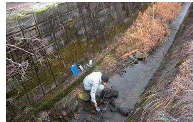
Contact of rainwater seeping underground with mineral ore may generate acid water that contains heavy metals. Monitoring water from surrounding springs is essential, even in a suspended and closed mine.
